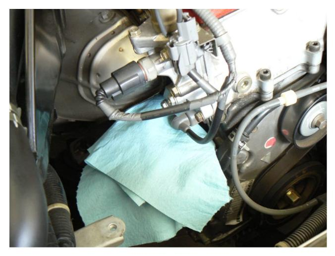
The TCT (outlined below) is held onto the engine with two 10 mm brass bolts (marked with red paint in the pic), and it has an inspection cover with two silver 10 mm bolts – be sure you loosen the correct bolts, mainly to save time. Use the 10 mm socket to loosen and remove the brass bolts.
