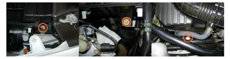
Before you can pull the airbox out, you have to detach three lines that are clipped to the back of the box, unscrew the sensor on top of the box, and detach the air hose that clips to the right side of the box. Use the photo below as reference – simply pull them loose. Once all the bolts are off and the wires are free, pull the airbox out and set it aside.
