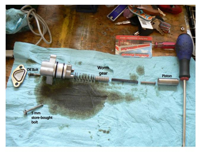
Remove the two 10 mm silver bolts from the TCT body and remove the cover plate. (far left part in the pic above) Unscrew the oil bolt from the body and place it aside for now.
