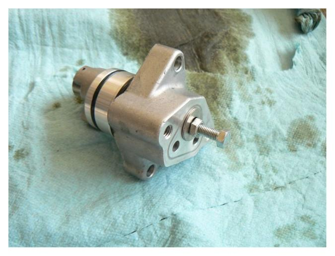
Apply a thin coat of oil to the o-rings. Push the TCT back into the engine – it will pop in and seat tightly. Reattach the TCT to the engine using the two brass 10 mm bolts. Torque to 8.7-9 lbft.
