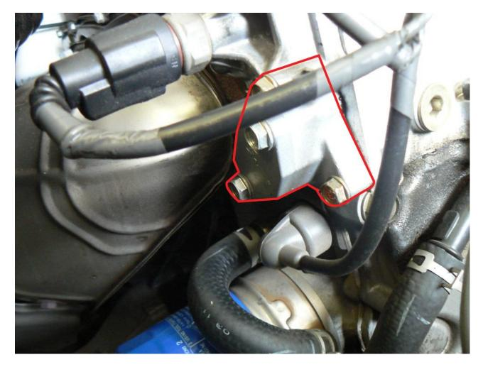
Once the bolts are off, you will need to pry the TCT out. It is tightly secured thanks to internal o-rings, so twist and pull to pop it off, but be careful about pulling too aggressively since you don't want to drop the assembly parts once you get the TCT out. Gently prying with a flathead screwdriver near where the 10 mm bolt goes can help – just be mindful not to damage the metal.
